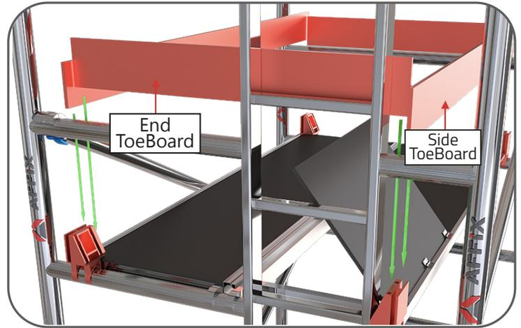
Then insert the **Side Toeboard** and the **End Toeboard** in the respective toeboard slots as shown in the figure.
